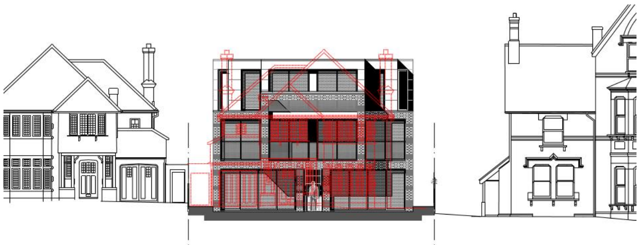
Proposed front elevation against existing building (red)
